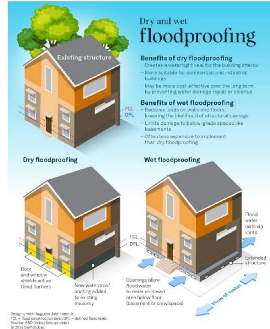
Figure 6: Dry and wet floodproofing
